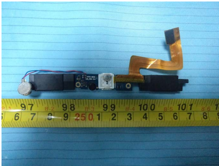
EUT – Sub Board Top View
