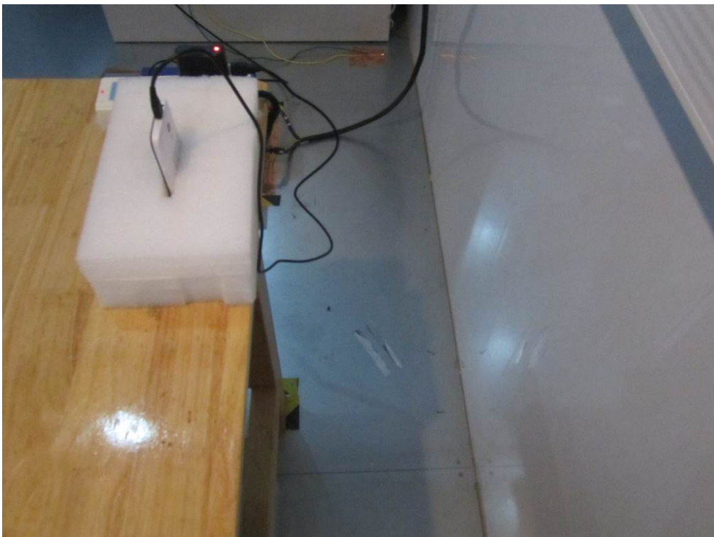
Conducted Emissions Test Setup Side View
