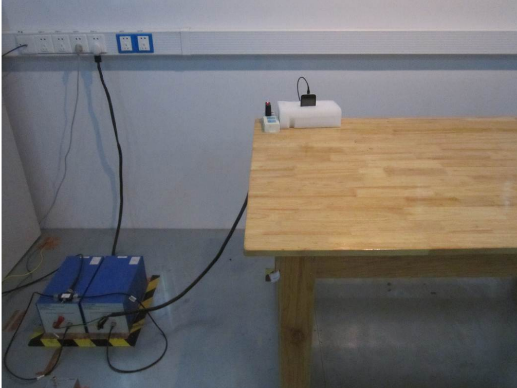
Conducted Emissions Test Setup Front View
