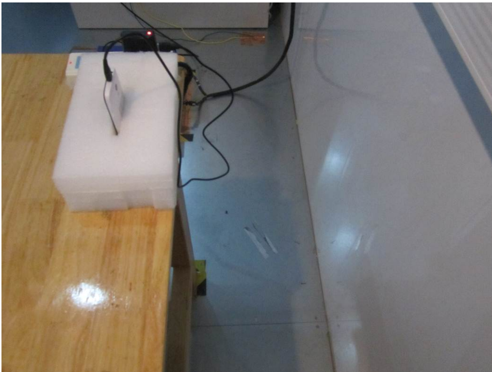
Conducted Emissions Test Setup Side View
