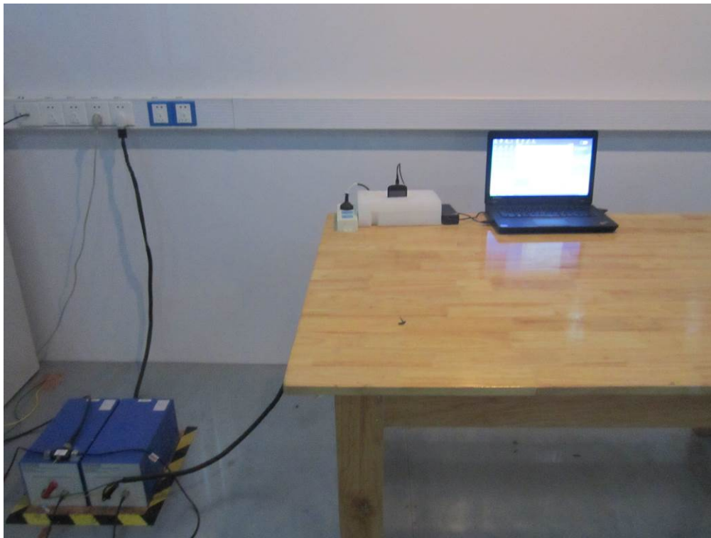
Conducted Emissions Test Setup Front View
