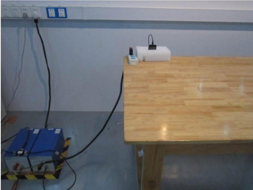
Conducted Emissions Test Setup Front View
