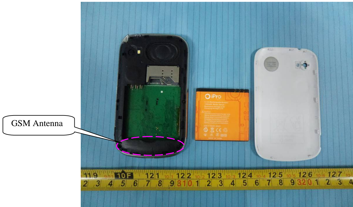
EUT – Battery off View
