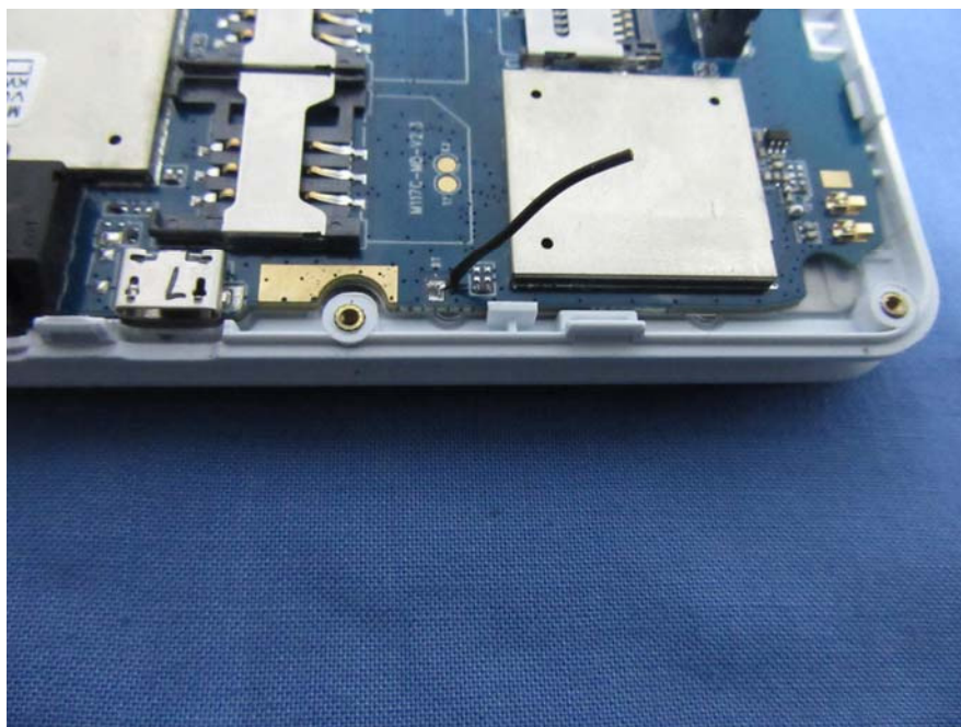
EUT – Bluetooth Antenna View
