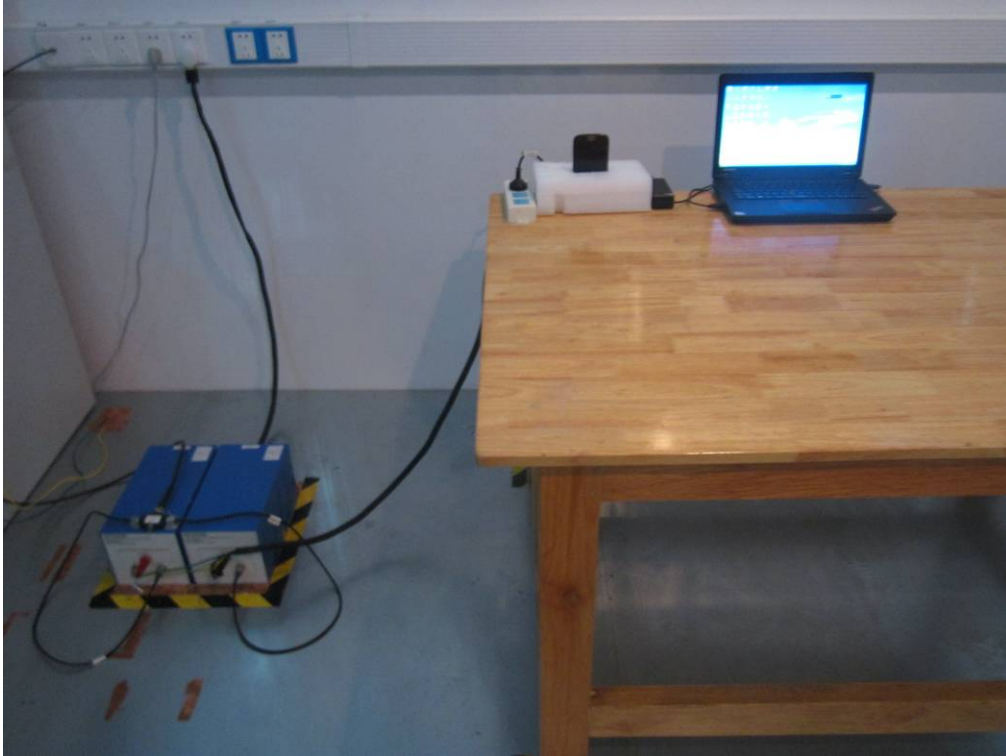
Conducted Emissions Test Setup Front View
