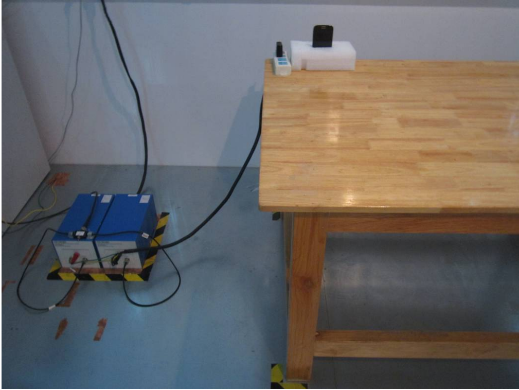
Conducted Emissions Test Setup Front View
