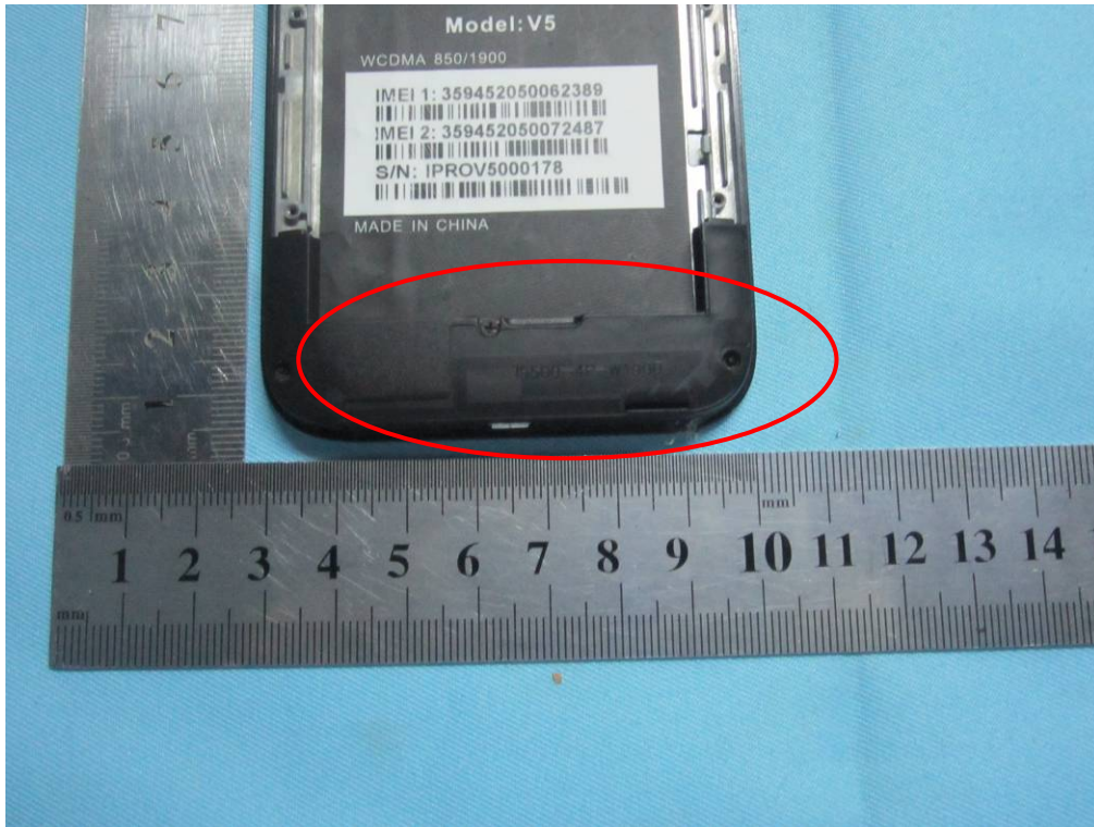
GSM / PCS/ UMTS Antenna View
