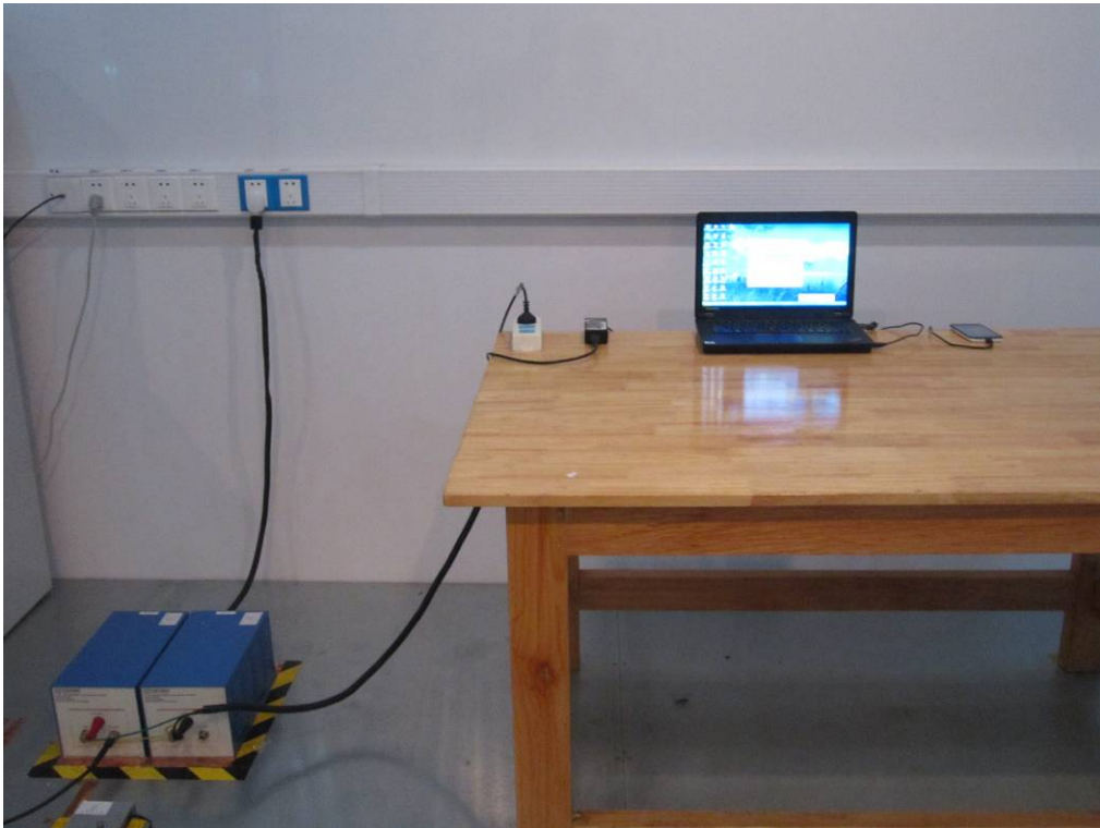
Conducted Emissions Test Setup Front View
