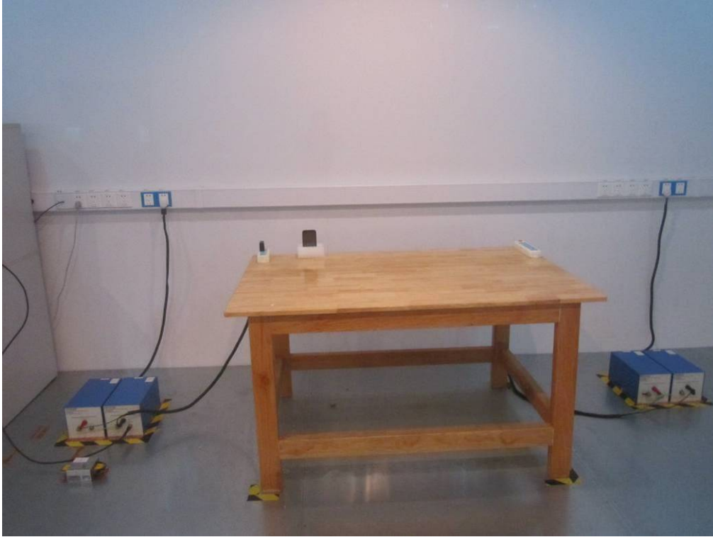
Conducted Emissions Test Setup Front View
