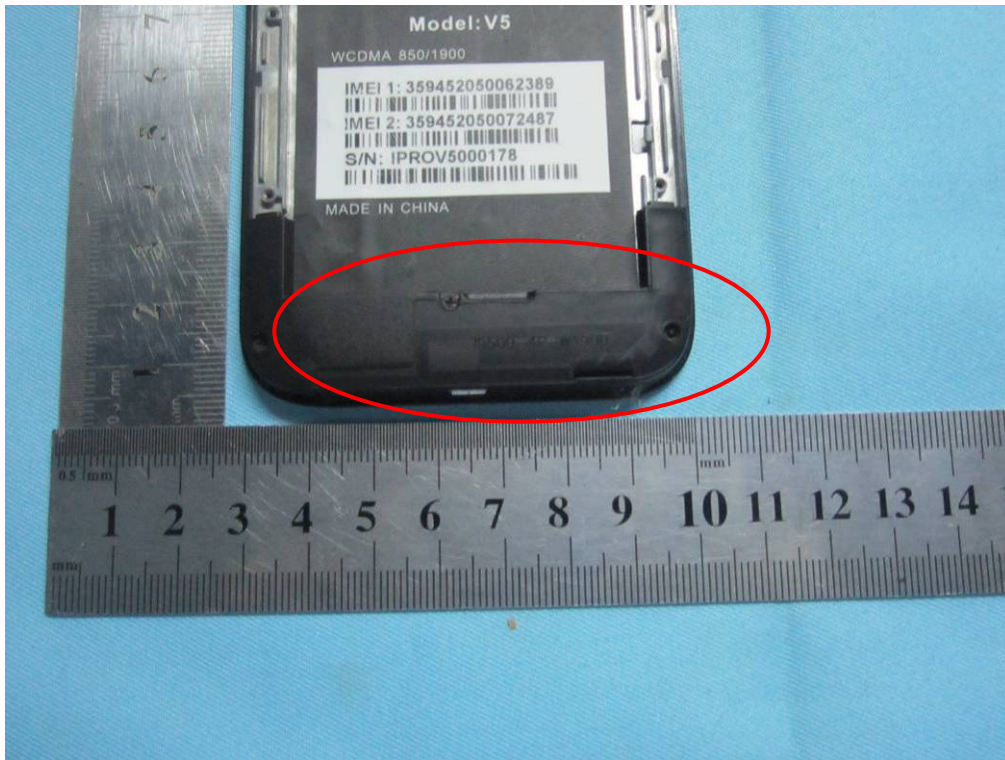
GSM / PCS/ UMTS Antenna View
