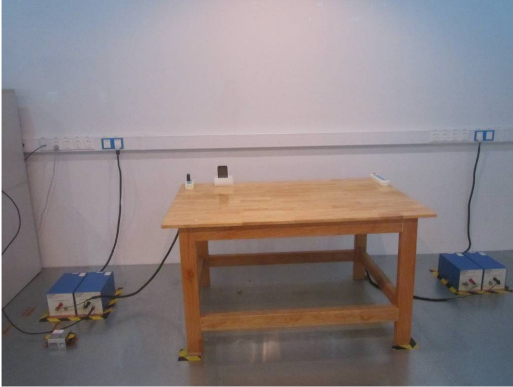
Conducted Emissions Test Setup Front View
