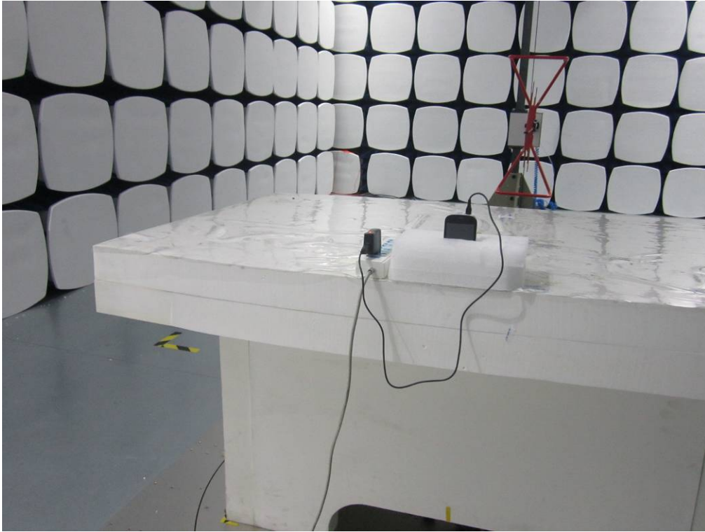
Radiated Spurious Emissions Test Setup Below 1GHz - Front View
