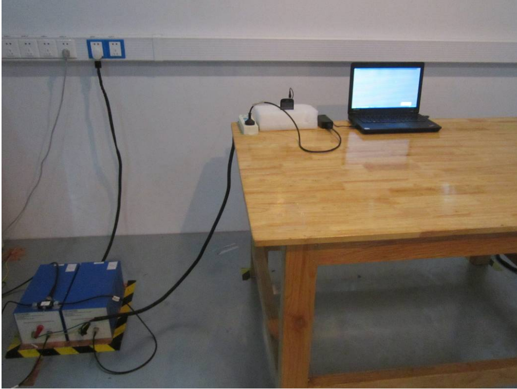
Conducted Emissions Test Setup Front View
