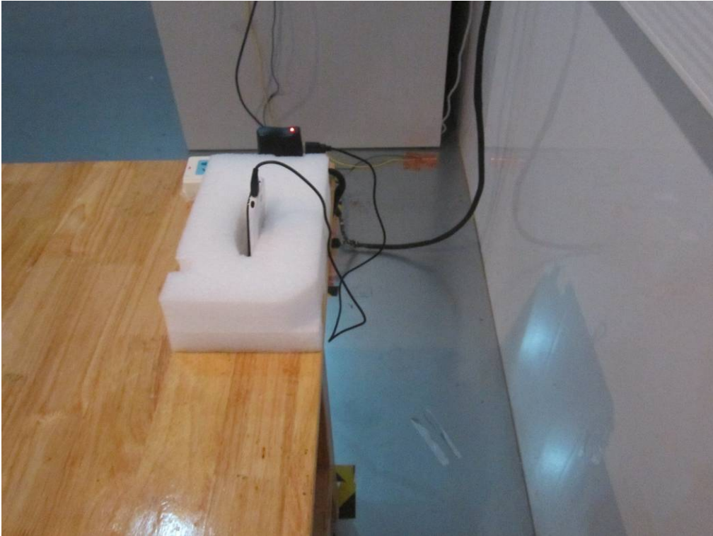
Conducted Emissions Test Setup Side View
