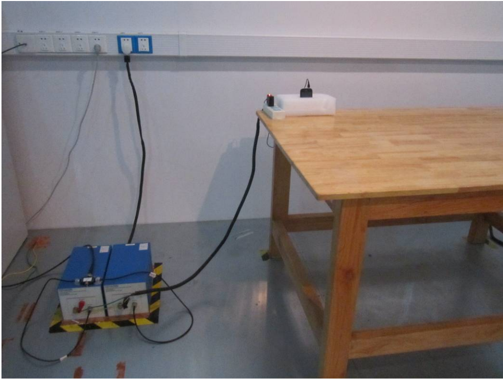
Conducted Emissions Test Setup Front View
