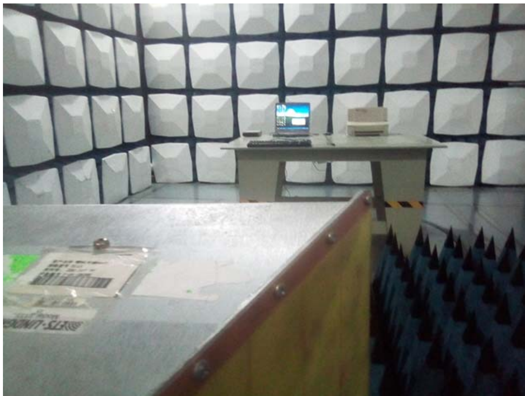
Radiated Emission Above 1GHz Rear View
