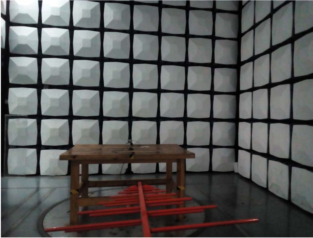
Radiated Emission Above 1GHz View
