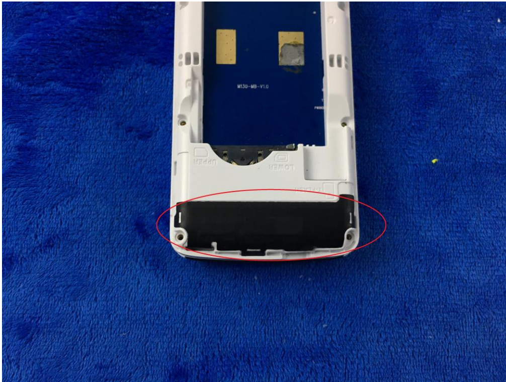
GSM/PCS Antenna View
