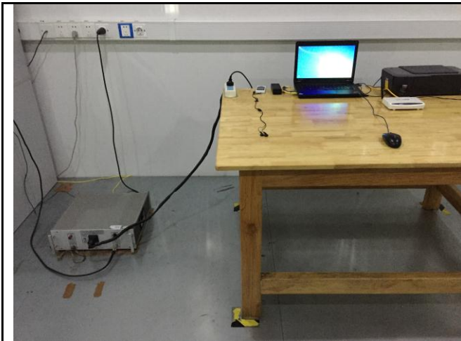
Conducted Emissions Test Setup – Front View
