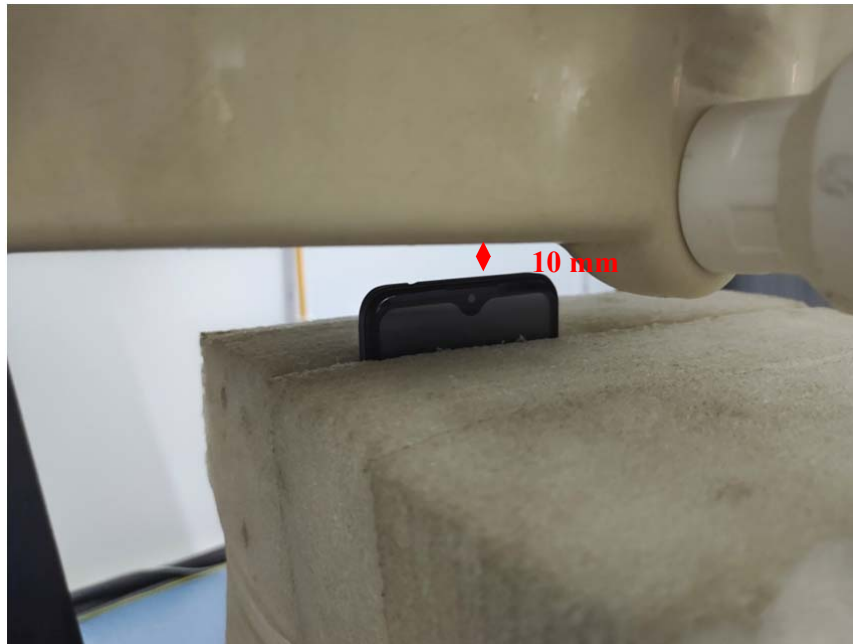
Body Bottom Setup Photo (10mm)
