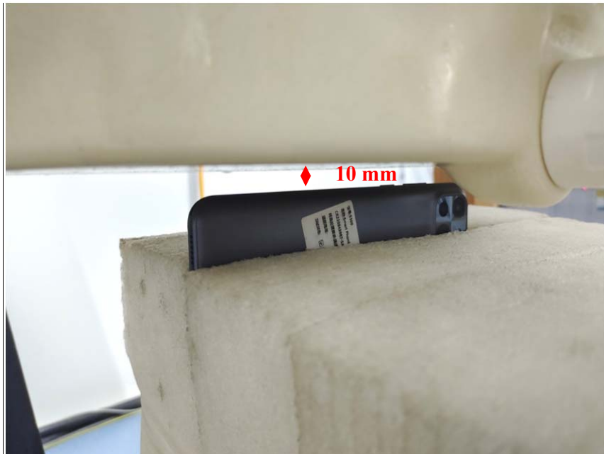
Body Right Setup Photo (10mm)
