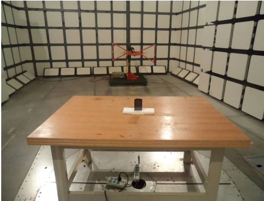
Radiated Emissions View (Below 1 GHz)
