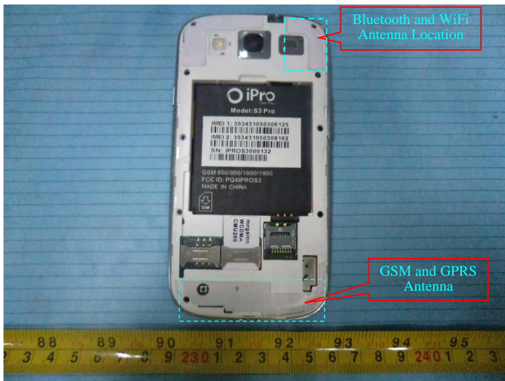
BT&WiFi and GSM Antenna Location:
