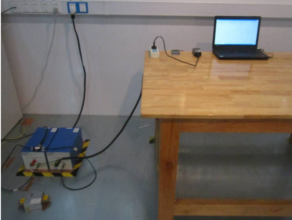
Conducted Emissions Test Setup Front View
