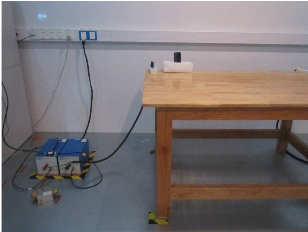
Conducted Emissions Test Setup Front View
