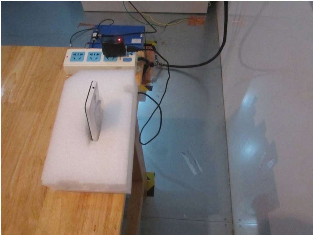
Conducted Emissions Test Setup Side View
