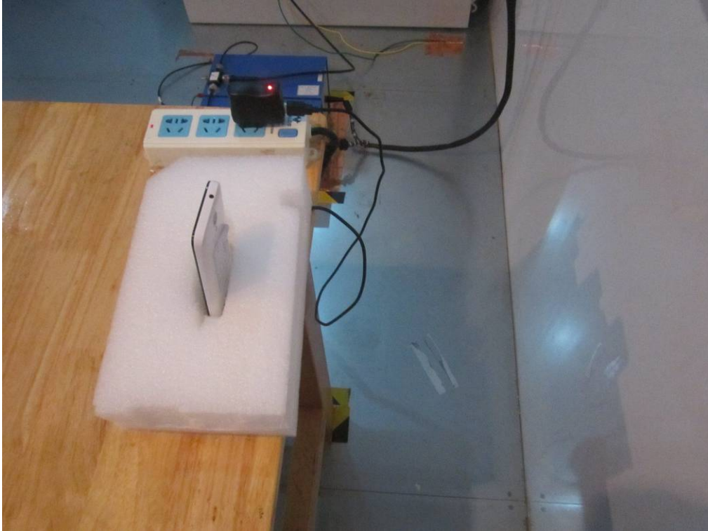
Conducted Emissions Test Setup Side View
