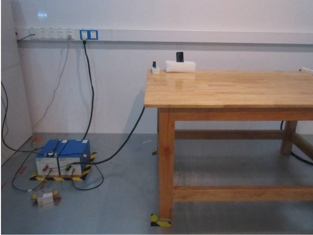
Conducted Emissions Test Setup Front View
