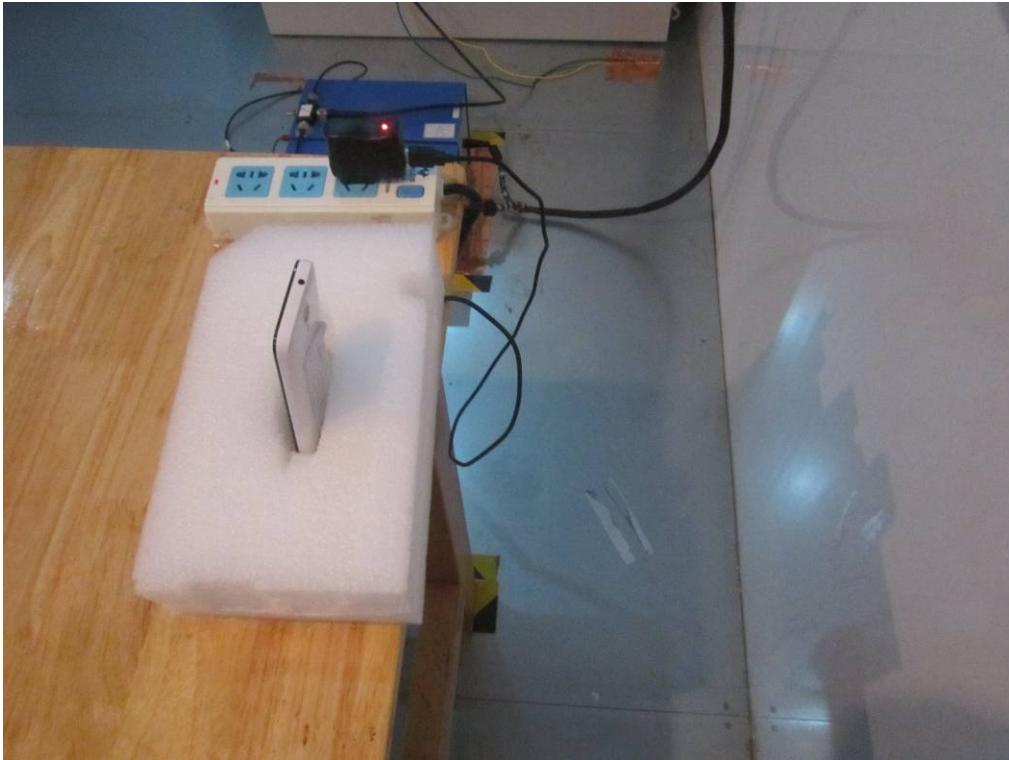
Conducted Emissions Test Setup Side View
