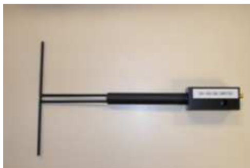
Figure 1 – Satimo COMOSAR Validation Dipole
