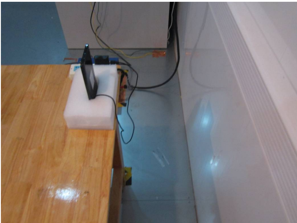
Conducted Emissions Test Setup Side View
