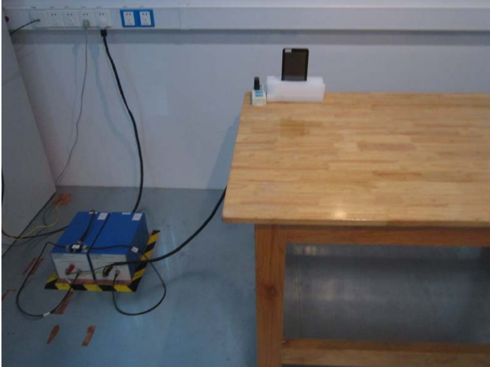
Conducted Emissions Test Setup Front View
