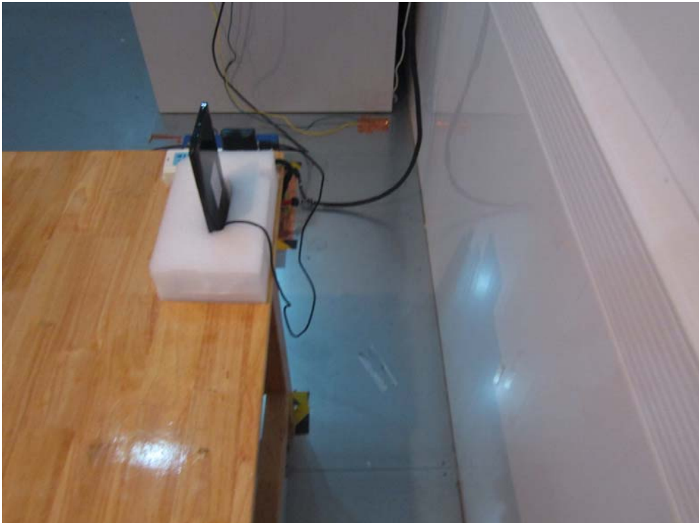
Conducted Emissions Test Setup Side View
