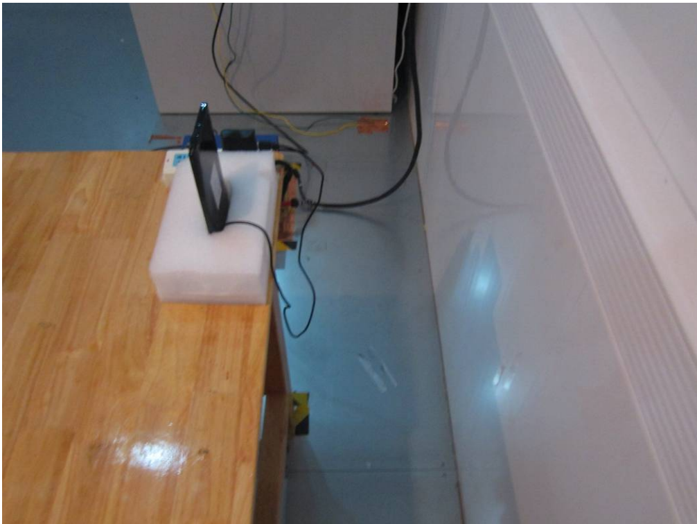
Conducted Emissions Test Setup Side View
