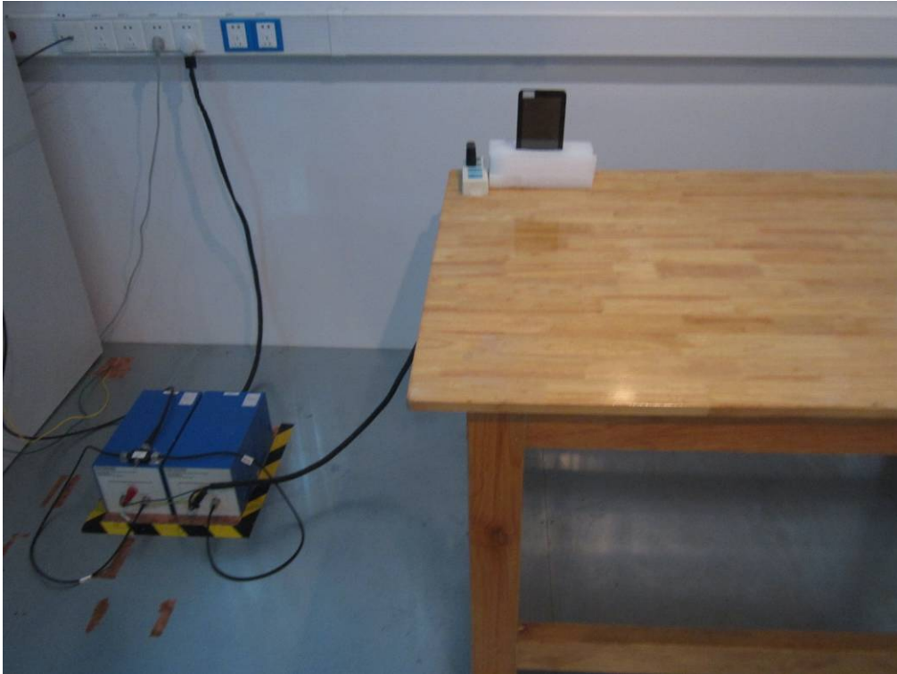
Conducted Emissions Test Setup Front View
