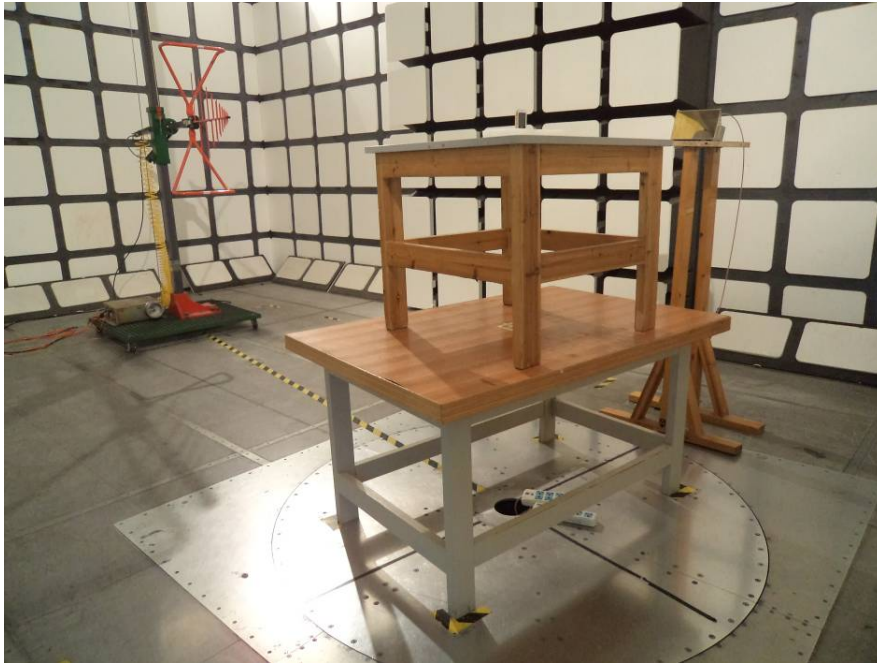
Radiated Emissions Test View – Below 1 GHz
