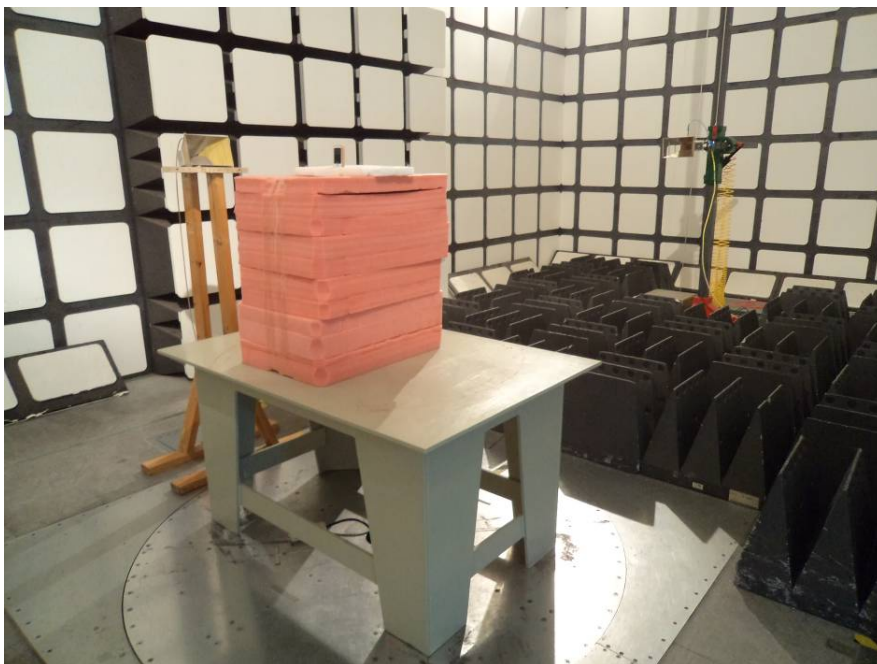
Radiated Emissions Test View – Above 1 GHz
