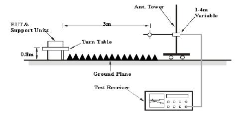
The radiated emission tests were performed in the 3 meters chamber test site A for the range 30MHz to 1GHz and the 3 meters chamber test site A for above 1GHz, using the setup accordance with the ANSI C63.4-2014. The specification used was the FCC Part 15.109 Class B limits.
