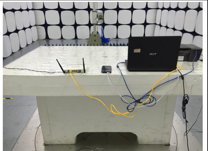
Radiated Emissions Test Setup Above 1GHz
