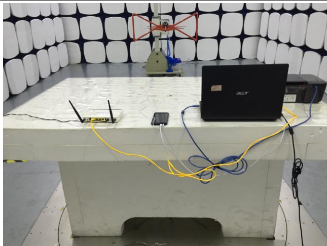
Radiated Emissions Test Setup Below 1GHz
