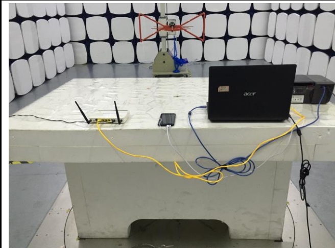
Radiated Emissions Test Setup Below 1GHz
