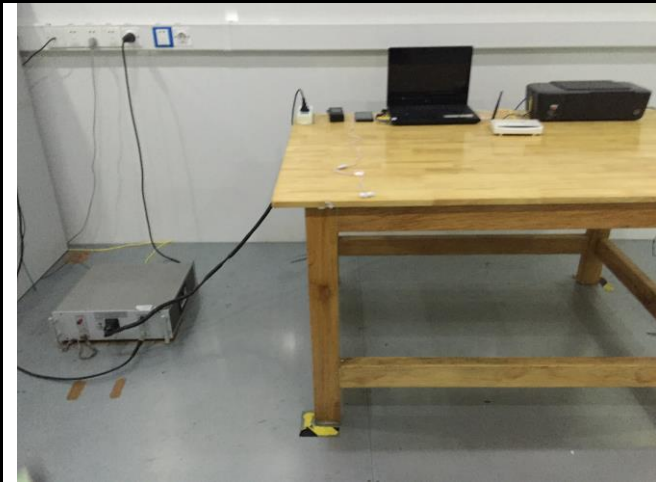
Conducted Emissions Test Setup – Front View
