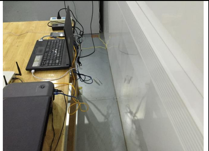
Conducted Emissions Test Setup – Side View
