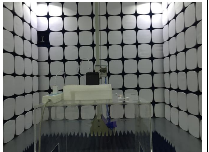
Radiated Spurious Emissions Test Setup Above 1GHz
