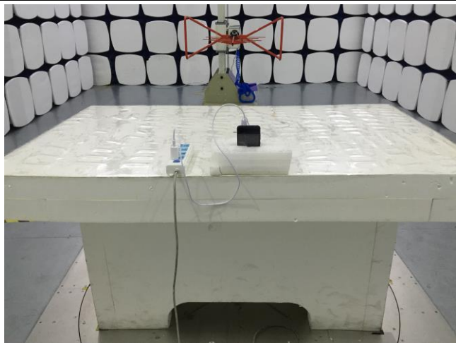
Conducted Emissions Test Setup Front View
