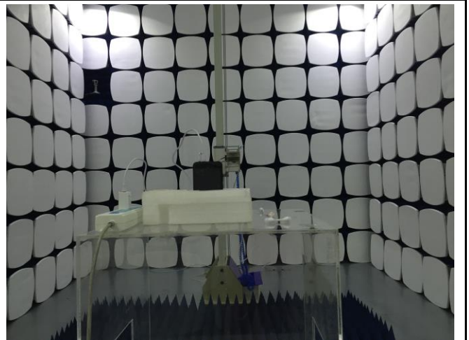
Radiated Spurious Emissions Test Setup Above 1GHz
