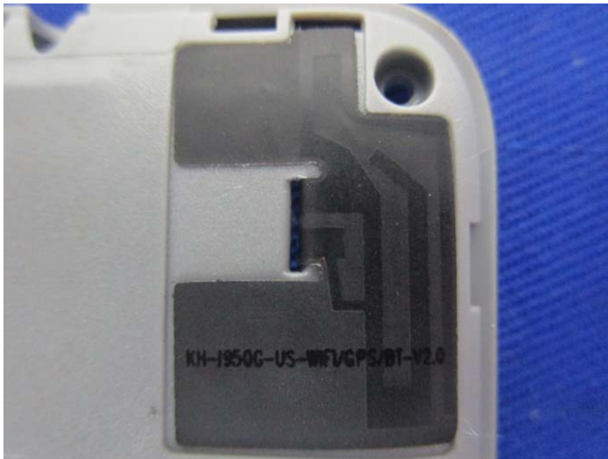
EUT- BT&WIFI Antenna View
