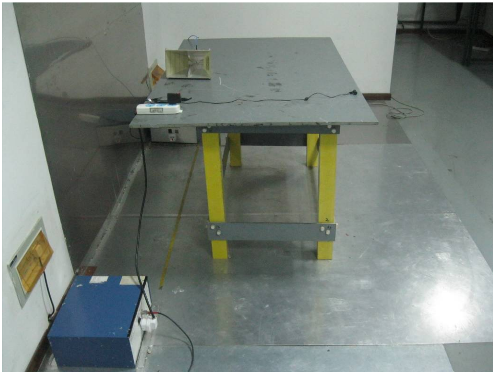
Conducted Emissions Test Setup - Side View
