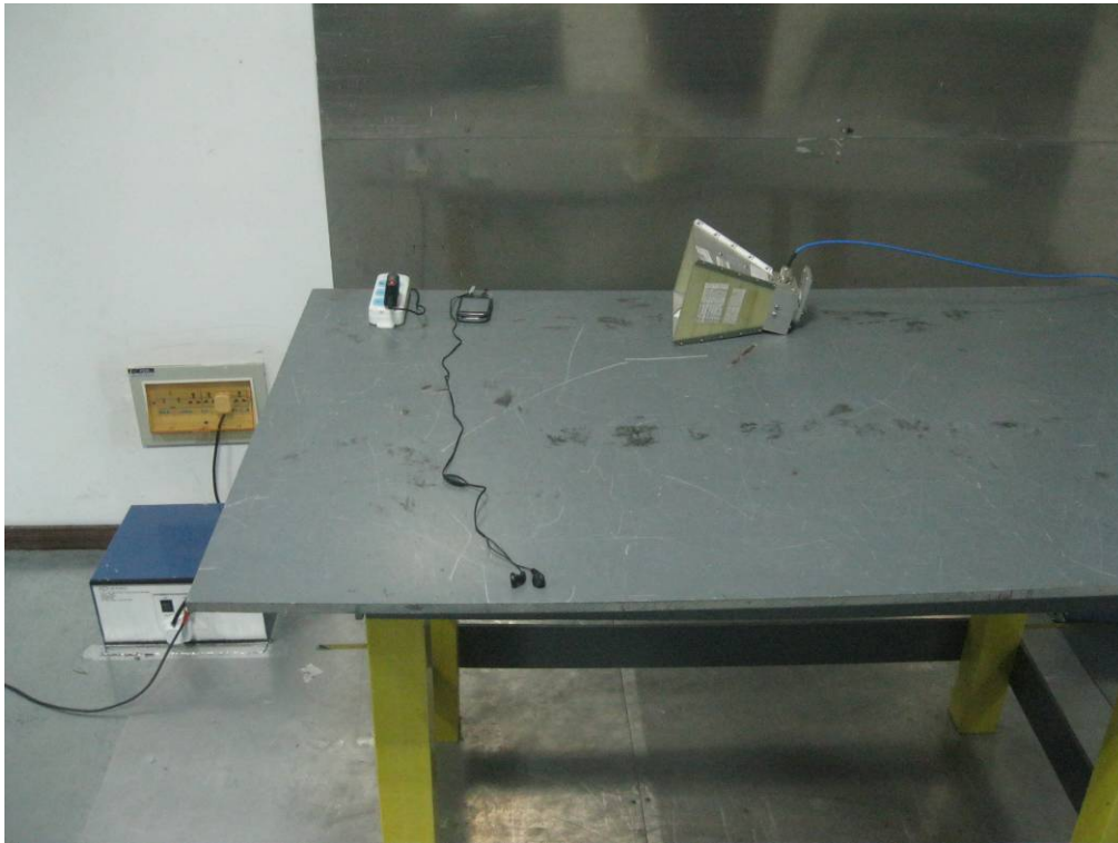
Conducted Emissions Test Setup - Front View
