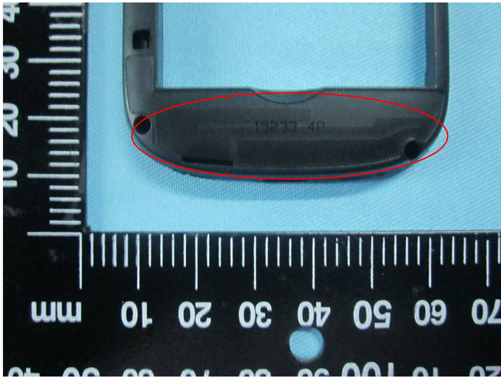
GSM/PCS Antenna View
