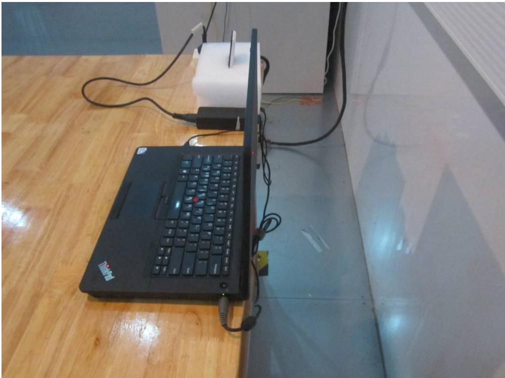
Conducted Emissions Test Setup Side View
