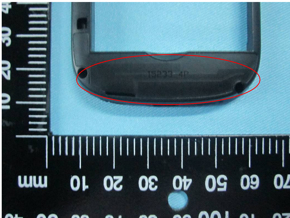
GSM/PCS Antenna View
