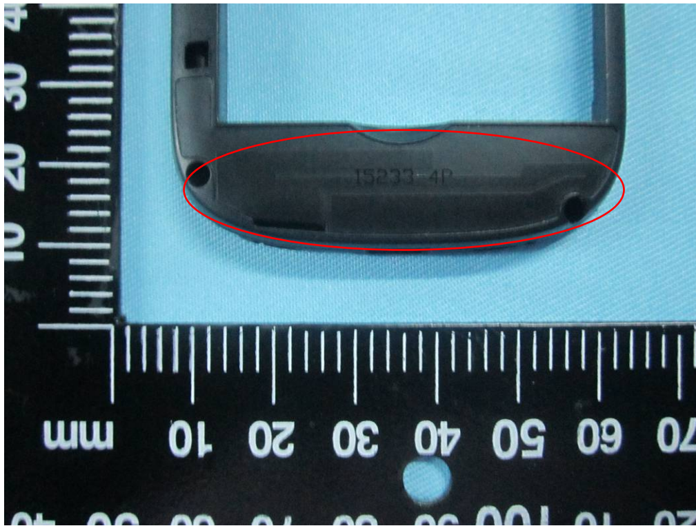
GSM/PCS Antenna View
