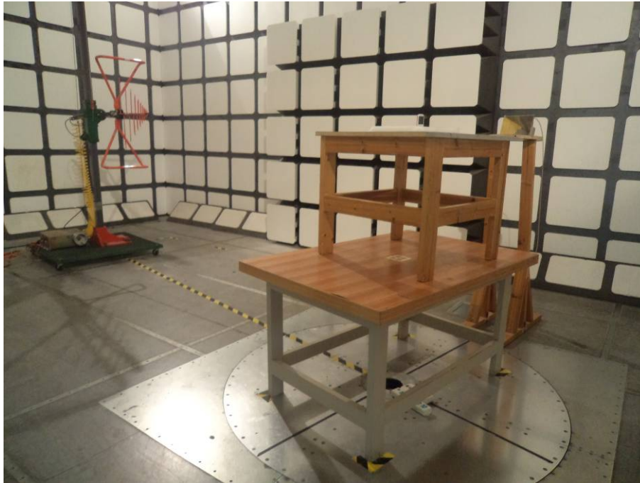
Radiated Emissions Test View (Below 1 GHz)
