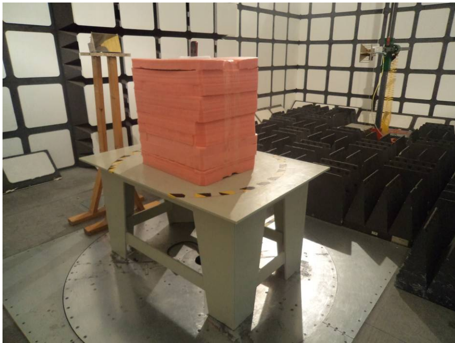
Radiated Emissions Test View (Above 1 GHz)
