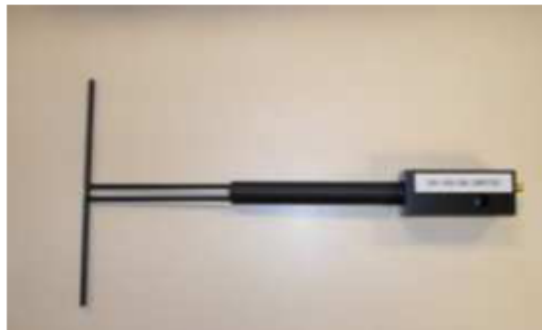
Figure 1 – Satimo COMOSAR Validation Dipole
