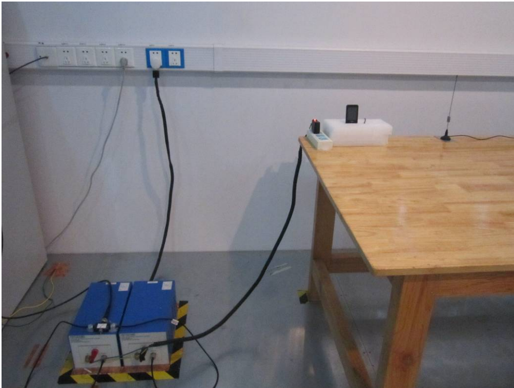
Conducted Emissions Test Setup Front View
