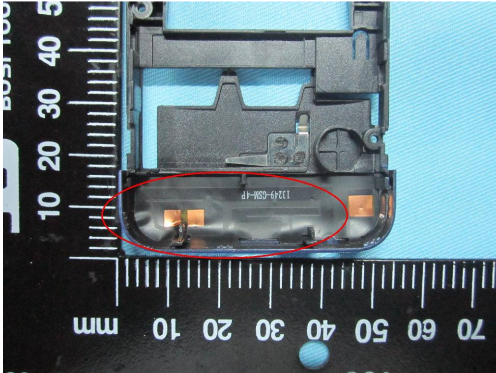
GSM/PCS Antenna View
