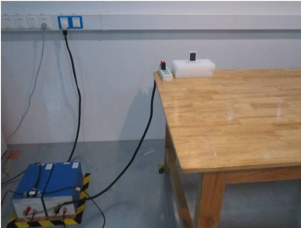
Conducted Emissions Test Setup Front View
