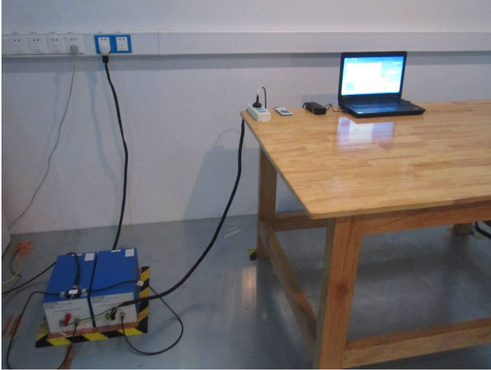
Conducted Emissions Test Setup Front View
